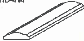
PROFILE OF HANDRAIL HD-414
