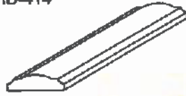
PROFILE OF HANDRAIL HD-414
