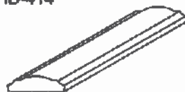
PROFILE OF HANDRAIL HD-414
