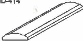
PROFILE OF HANDRAIL HD-414
