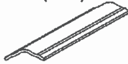
PROFILE OF HANDRAIL HD-514 (HOLO)
